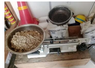
Figure 2.2 Equipment and materials for sand cone testing in the laboratory
