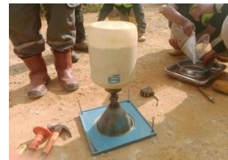
Figure 2.1 Equipment and materials for sand cone testing in the field
